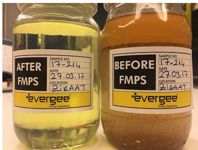
Right-before fuel polishing, Left- after fuel polishing
